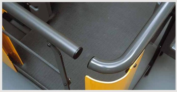
The protective rail has a contoured, well moulded design. It will bear a load of 90 kg. The safety gates are optional below 3 metres. The floor is floating, i.e. vibration-damping, and comfortable to stand on. No pedals. Flat, uncluttered surface.
