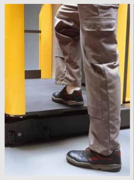
Low step in. Clear entry with the foot protector attached to the gate, giving protection when the gates are lowered.
