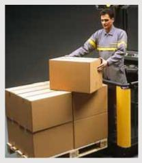
The Atlet Ergolift is the independent fork lift for the picking pallet. Always at the right height for setting down. The lift unit takes very little space and does not interfere with the layout of the cab. Lift capacity 1000 kg for all models.
