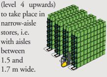
The trucks are then rail or wire guided, passing through the aisle without the driver needing to steer.
