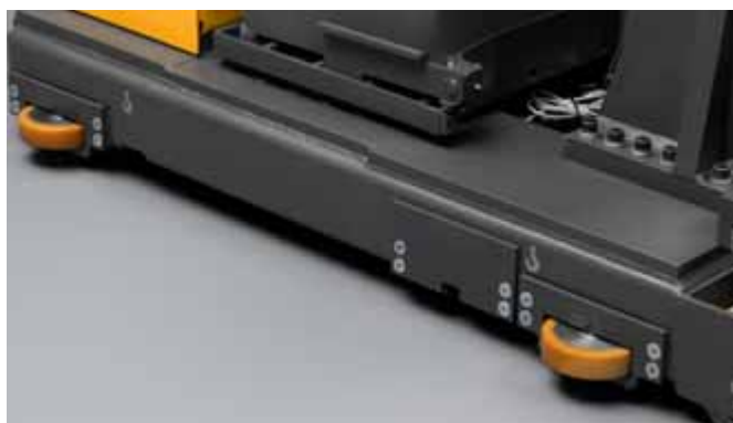
Complete package for rail- or wireguided steering.
