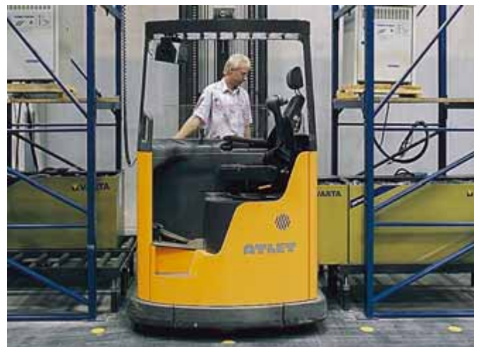
Powered battery change for multi shift operation.
