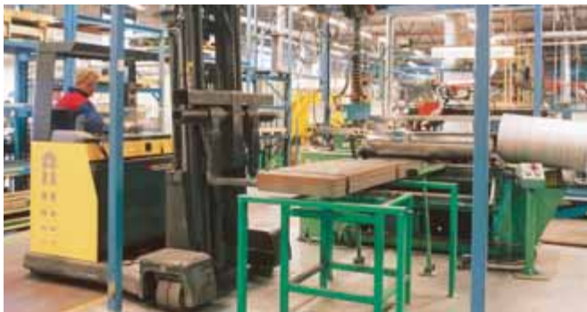
Smooth production supply. From warehouse to machine with one truck with its compact dimensions Atlet's four-way truck is as easy to manoeuvre as an ordinary reach truck.
