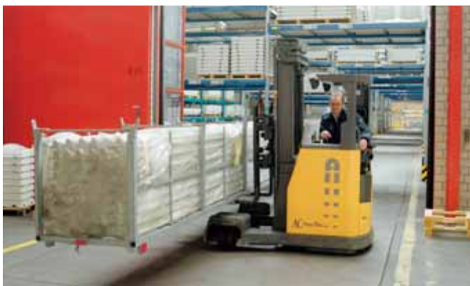
When traveling sideways the driver has a good view of the goods and the working area. Sideseated driver provides best ergonomics when driving sideways.
