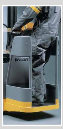
The driver's platform comes in two versions with either a folding side restraint or a permanent protective guard that gives a relaxing position for long cycles.
