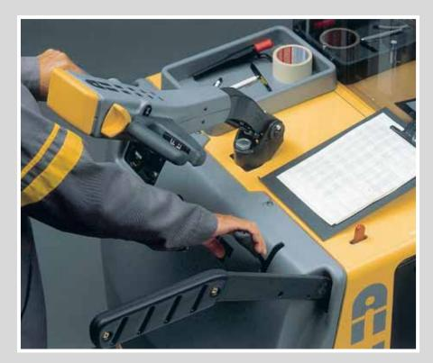
The lifting movement is controlled by a slide valve with the control unit comfortably placed to the right of the tiller arm and giving fingertip precision.
