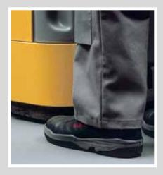
Foot injuries are no longer possible since the NOVA has such a low chassis that feet or rather safety shoes cannot get beneath it. Castor and drive wheel are both retracted. If the truck makes contact with a foot it just pushes it out of the way.
