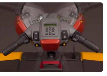
The steering of the future is here. Atlet's new Ergo steering handle controls all the functions from one place. The handle is designed to reduce movement and therefore minimize the strain on the driver.
